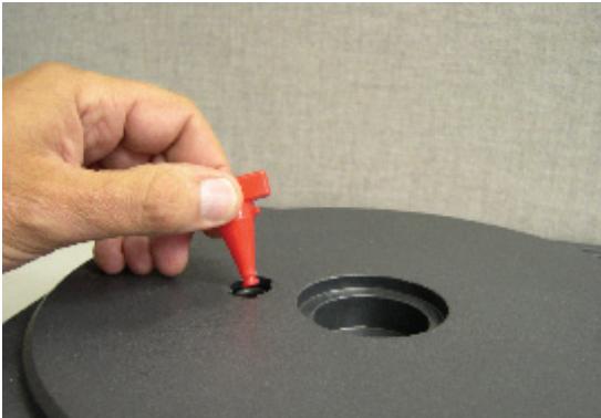
Figure 9: Remove red plug before loading
