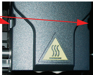
Figure 18: Removing the Head Cover
